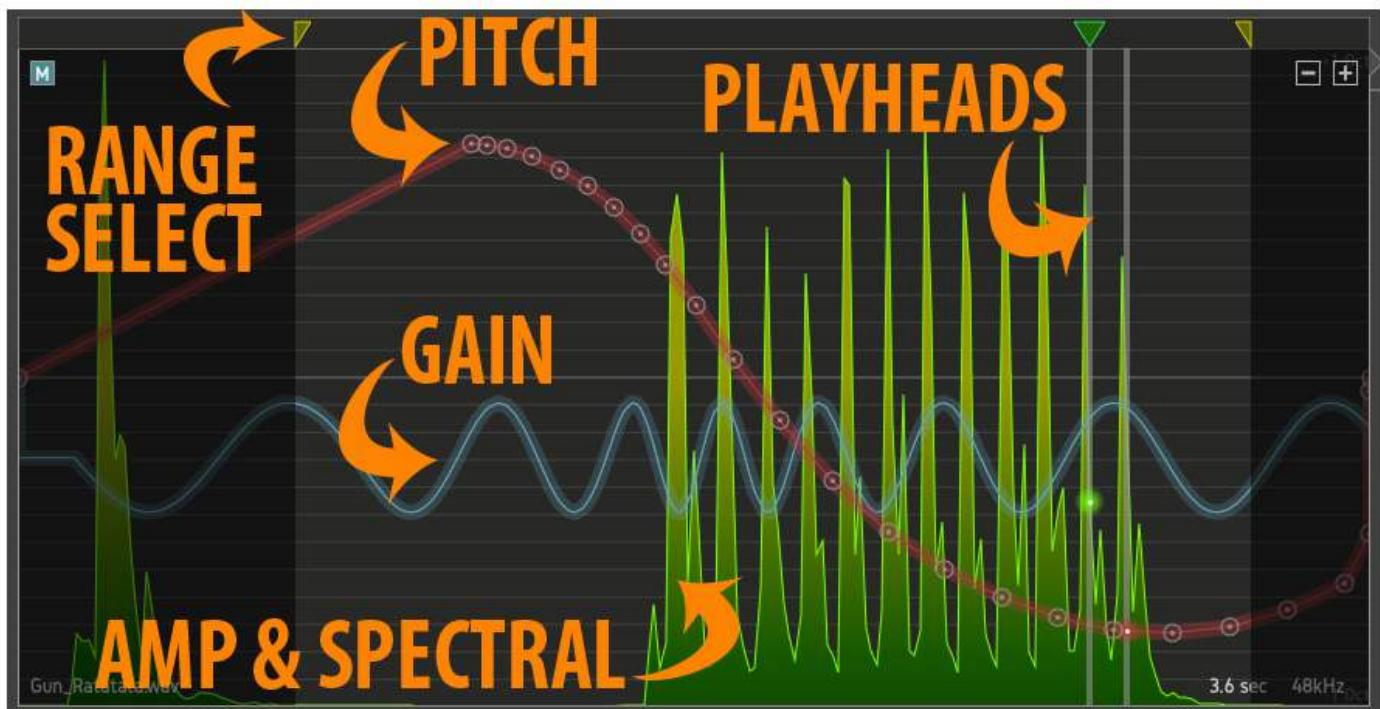
**The Pitch and Gain lines** use the colour corresponding to their process module and their respective Edit Mode buttons. Pitch is red or orange, gain is blue. The Amplitude envelope is represented by the bright green outline, whereas the Spectral envelope is represented by the green/yellow fill colour. When a module is turned off, its envelope path will become "greyed out".
