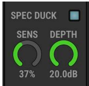
DEPTH controls the maximum cut that may be applied to any one frequency.
